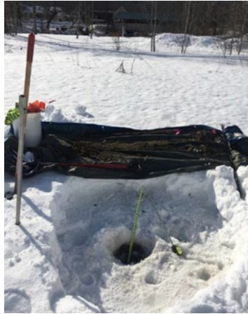
Figure D20. A hand auger and shovel were used to assess soil conditions and infiltration potential.
