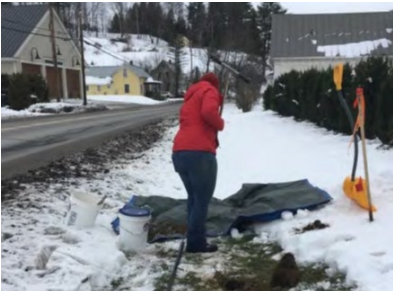
Figure C17. A hand auger was used to assess soil conditions and infiltration potential.
