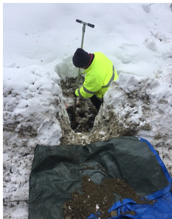
Figure A21. A hand auger and shovel were used to assess soil conditions and infiltration potential.
