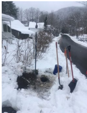
Figure E25. A hand auger and shovel were used to assess soil conditions and infiltration potential.
