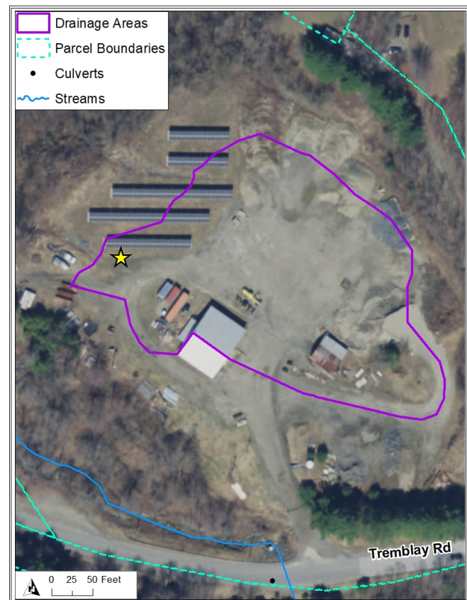
Figure D14. The proposed BMP drainage area is shown in purple. The recommended BMP locations are shown with stars.
